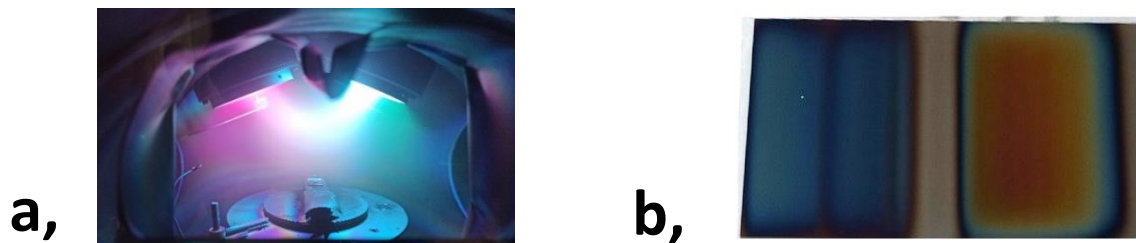
Figure 1: a , Reactive burst HiPIMS sputtering of Y (left) and Ti (right) b , resulting combinatorial Y_xTi_{1-x}O_y sample
