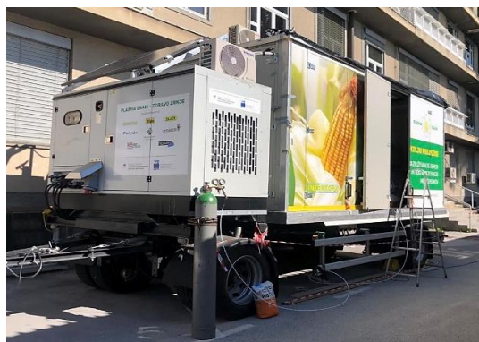
Figure 1. Mobile plasma reactor for seed treatment.
